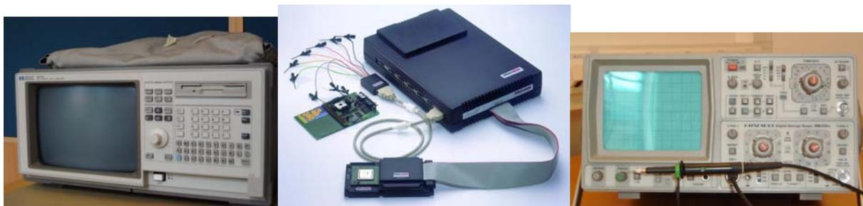
Figure 2.3: A logic analyser, an emulator and an oscilloscope
